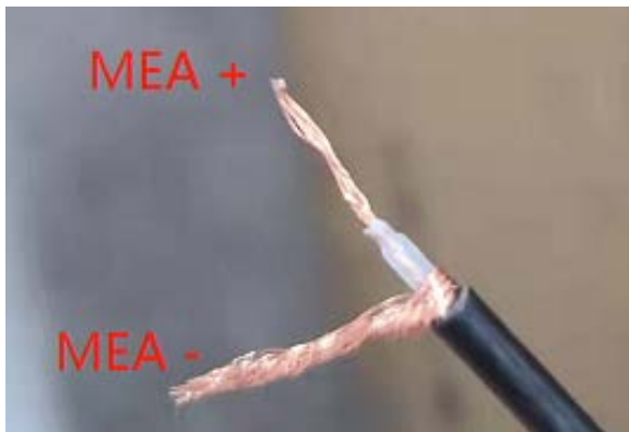
Sensor wire - Terminal : "+" and "-"
